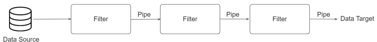
Figure 16. Pipe and filter pattern scheme.
